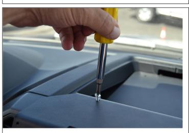
4. Attach the ProClip mount by inserting the included screws into the holes and threading them into the existing threaded holes in the dash.
