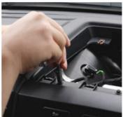
1. Remove the rubber pad on the bottom of the upper dash tray.
