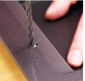
3. Place the ProClip mount into the dash tray. Mark the two front holes with a pencil. Take the ProClip mount out of the tray and then drill two holes in the tray where the marks have been made.
